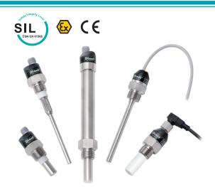
Capacitive level sensors (switches) CLS–23 are designed for limit level detection of electrically conductive and non-conductive liquids in vessels, reservoirs, sumps, pipes, tanks, etc. The sensitivity of the sensor can be easily set by placing magnetic pen on sensitive spot.
